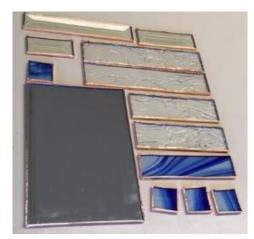
Once you have chosen your glass components, pieces are cut and foiled. In this picture, three bevels, box sides and ends, box bottom (mirror), and four variegated blue pieces have been prepared. The bevels and the four blue pieces are for the top of the box.
