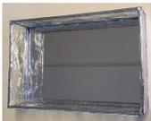
The basic box is constructed. Each piece is foiled, then soldered together.
